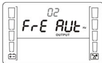
Figure 5-3 Setting the system output frequency
