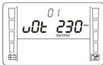
Figure 5-2 Setting the output voltage
