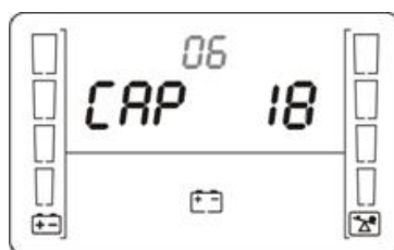
Figure 5-4 Setting the battery capacity
